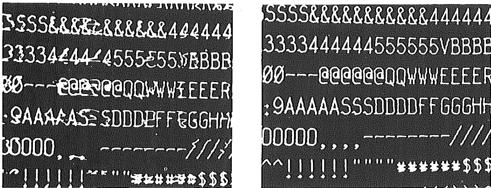
Figure 6.18. Effect of “glitches” on a display.
